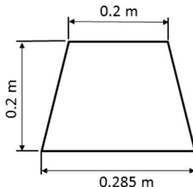
Fig. 1. Cross-section of the idealised concrete sleeper.
