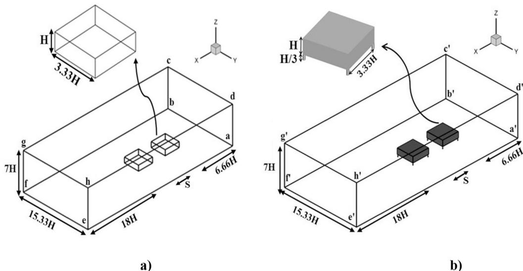
Fig. 1. Computational domain for inline buildings, a) Standard buildings, b) Supported buildings.
