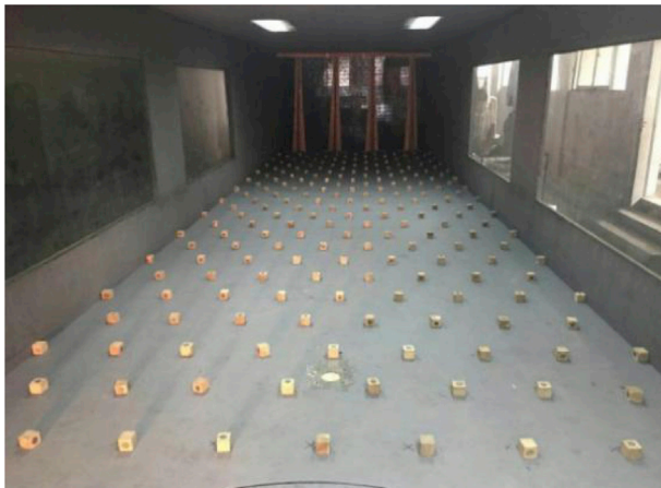
Fig. 4. Simulation of the turbulent wind field in the wind tunnel.
