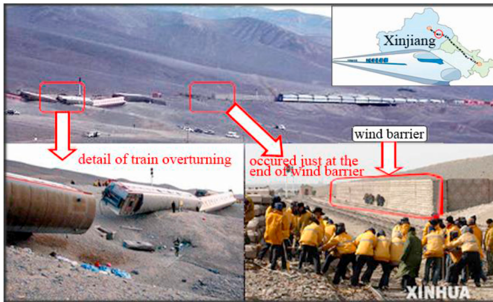
Fig. 1. Train overturning induced of variations of aerodynamic loads around wind barrier.
