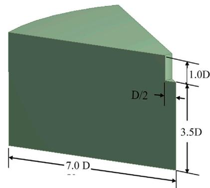
Fig. 1. Numerical geometry and dimension for downburst domain.
