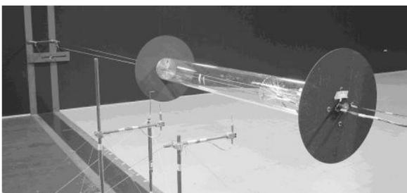
Fig. 2. Rigid model installed in the wind tunnel test section (Belloli et al., 2005b).
