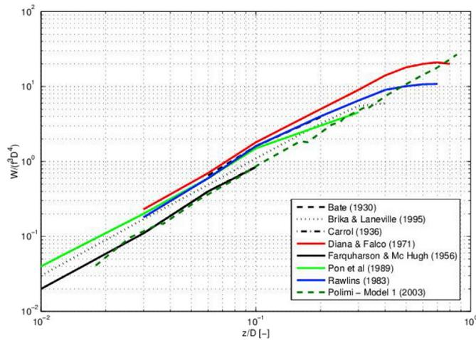
Fig. 1. Specific power input as function of vibration amplitude (Transmission Line, 1979).
