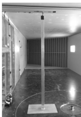
Fig. 1. Vertical experimental set-up installed in the test section (left) - Coil/magnet assembly (right).
