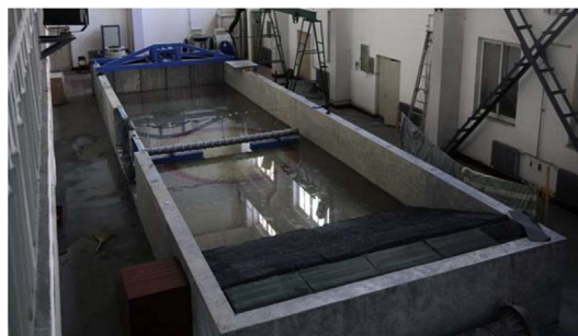
Fig. 1. View of the Earthquake, Wave and Current Joint Simulation System.
