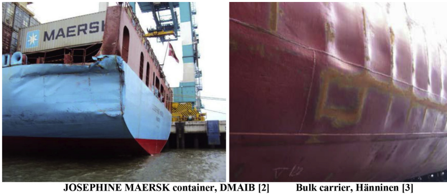
Fig. 1. Collision (left) and ice-contact (right) damage [2,3].
