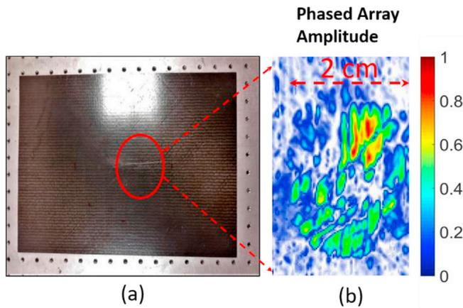
Fig. 1. Top view the CFRP sample (a), ultrasonic phased array images of the impact damage based on normalised amplitude measurements (b). As it can be seen from figure (b), the damaged region has a circular shape.
