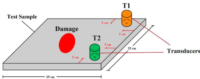
Fig. 2. CFRP test sample and location of transmitter transducers. T1 and T2 correspond to the Panametrics X1020 and the Piezoshaker PS-X-03-6/1000 transducers, respectively.
