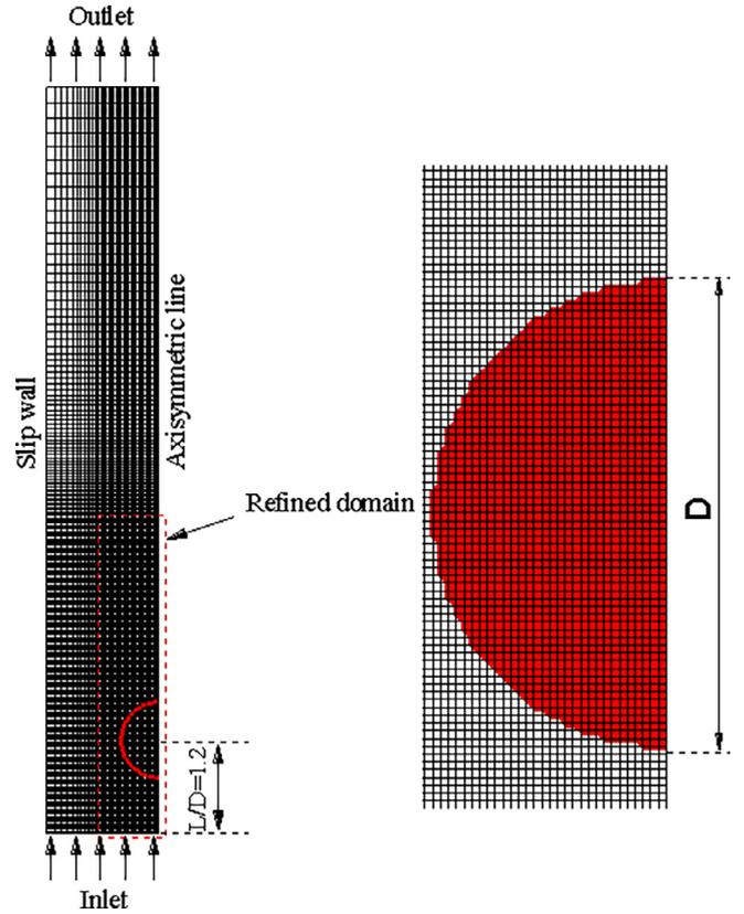
Fig. 1. Computational domain for bubble simulation.
