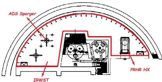
Fig. 1. Schematic of IRWST and PRHR HX.
