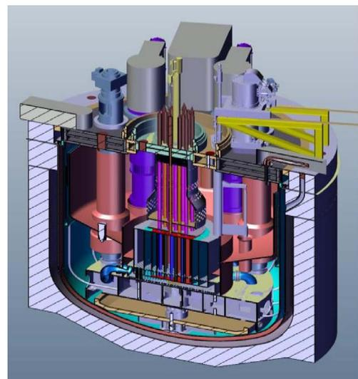
Fig. 1. Primary system arrangement for ASTRID.
