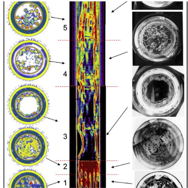
Fig. 3. Radiography and tomography of test bundles (Barrachin et al., 2013).
