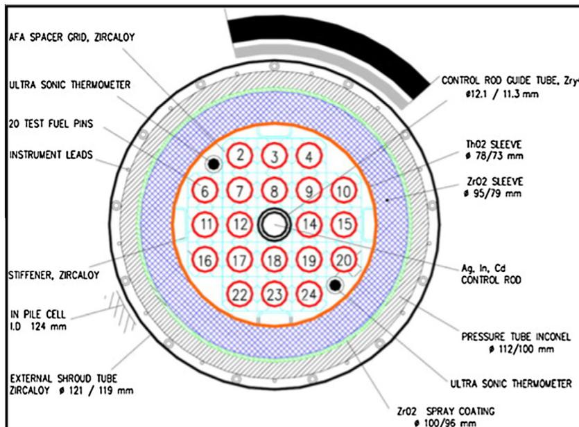
Fig. 2. Fuel assembly scheme (March and Teisseire, 2013).
