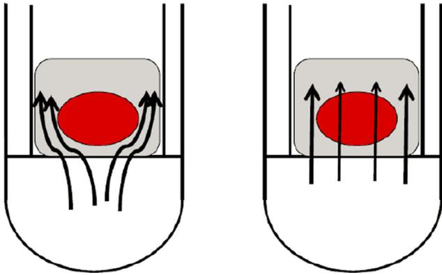
Fig. 1. Flow blockage model of MAAP and MELCOR (Wachowiak, 2014).
