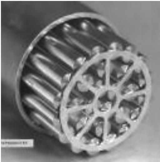
Fig. 1. Image of a 28-element bundle in pressure tube.
