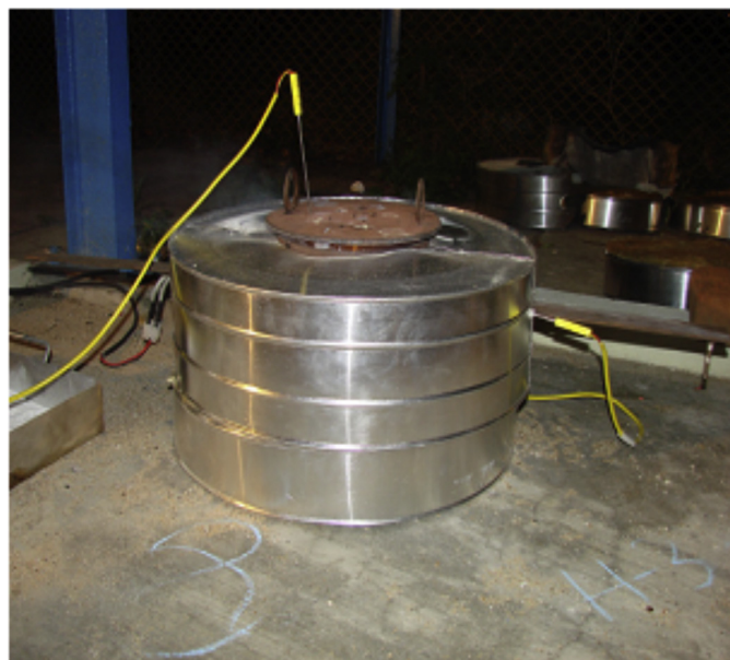
Fig. 2. Sodium exposure setup; CS vessel with thermal insulation using 150 mm glass wool associated with aluminium cladding.
