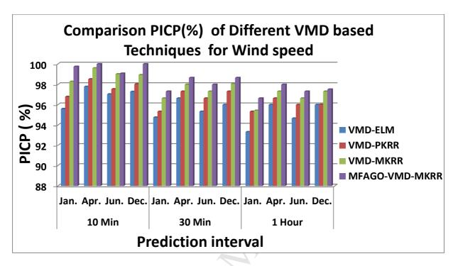
Bar graph comparison of PICP (%) for different VMD based hybrid techniques with the proposed MFAGO-VMD-MKRR for 10 min , 30 min and 1 hour interval wind speed at 95% confidence level
