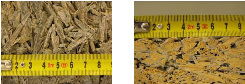
Fig. 2. (a) Timber-cement board – detail (b) cross section
