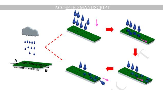
Film-type converters are made to harvest rain energy by PANi or PANi-graphene complex composite films, achieving maximum current and voltage of  $3.80 \mu$ A/droplet and  $85.01 \mu$ V/droplet, respectively.
