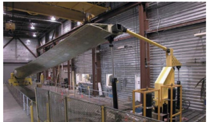
Fig. 2. Dual axis blade testing machine [18].
