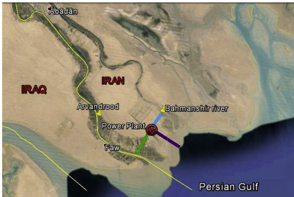
Fig. 1. Scheme of osmotic power plant in Bahmanshir. Dark blue arrow indicates salt water, pale blue arrow indicates freshwater and green arrow is the indicator of output water. (For interpretation of the references to color in this figure legend, the reader is referred to the web version of this article.)
