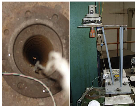
Fig. 2. Optical borehole deformation observation instrument.
