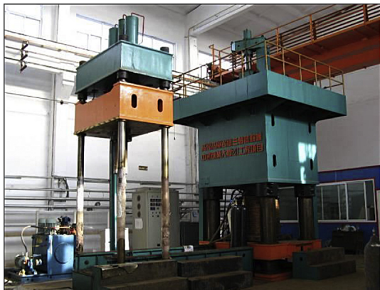
Fig. 1. 20 MN servo-controlled triaxial rock testing machine.
