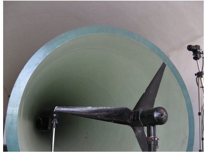
Fig. 1. B1/K2 wind tunnel and the wind turbine.
