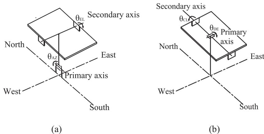
Fig. 1. Comparison of tracking schematics of: (a) pseudo-azimuthal mounting; (b) declination-clock mounting.
