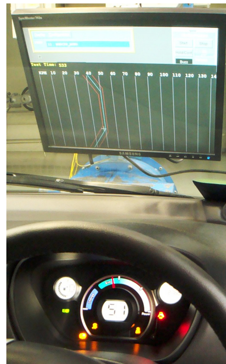
Fig. 2. Computerised driving aid for a human test driver to follow a predefined drive cycle used during the testing at Orbital's facility. The blue line in the centre of the track is the indication of required speed to be driven. The red lines show the driver the maximum allowed speed deviation for a valid test drive, and the crosshair is the present speed. The uncertainty of the results can be inferred by the difference between the speed reading on the dashboard (51 km/h), and the crosshair (~49 km/h) (For interpretation of the references to color in this figure legend, the reader is referred to the web version of this article.).
