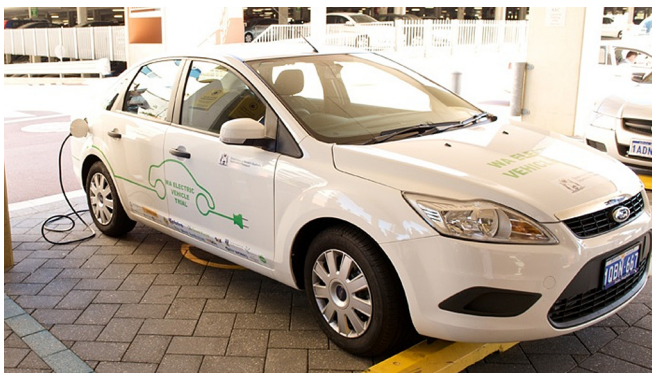
Fig. 1. The licenced Ford Focus converted to an EV that was used in the research. Source: Ref. [37].
