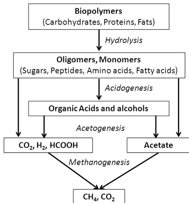
Fig. 1 – Steps of the biogas production process.
