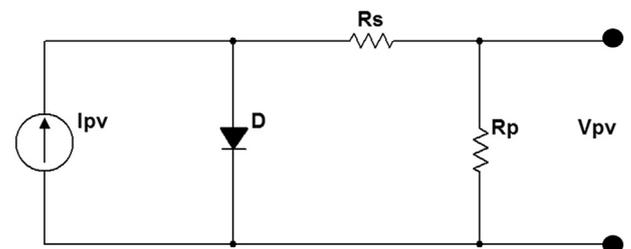
Fig. 1. Equivalent circuit for general PV cell model.
