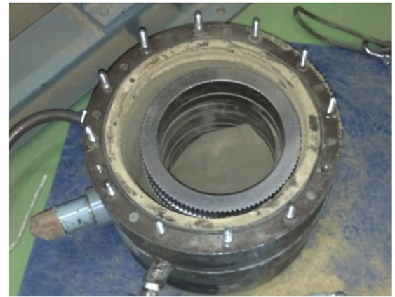
(a) Interior of the mill chamber
