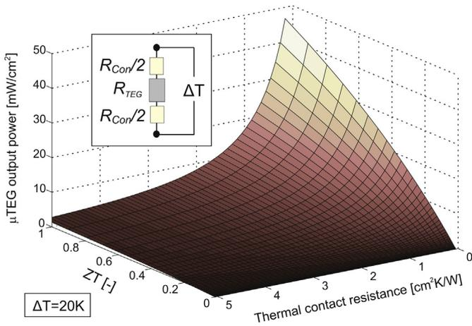
**Fig. 1.** Simulated output power of a 215 μm thick Bi<sub>2</sub>Te<sub>3</sub> μTEG ( $R_{TEG} = 2.8 \text{ cm}^2\text{K/W}$ ) in dependence of the ZT-value and the thermal contact resistance  $R_{Con}$  at an applied temperature difference of 20K. The simulations were performed applying a thermoelectric model under matched electrical load [17].
