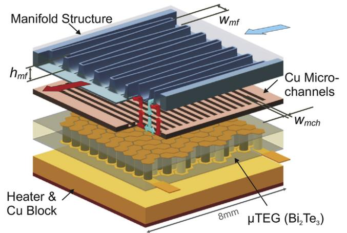
**Fig. 2.** Exploded view of the μHTS/μTEG system.
