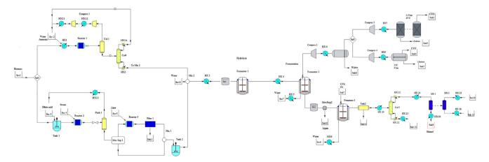
Fig. 1 – Superstructure of for the simultaneous production of ligno – i-butene and lignocellulosic based ethanol.
