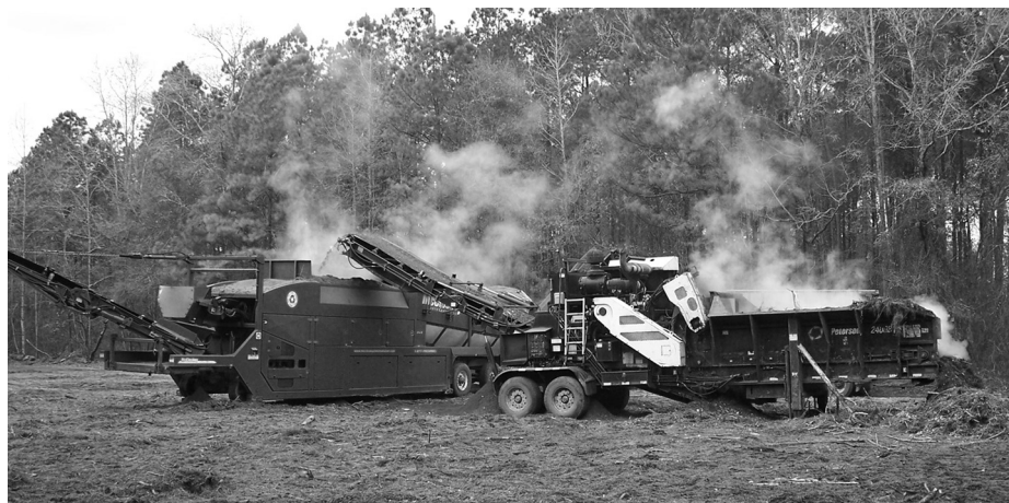
Fig. 1 – Trommel screen fed by a horizontal grinder.
