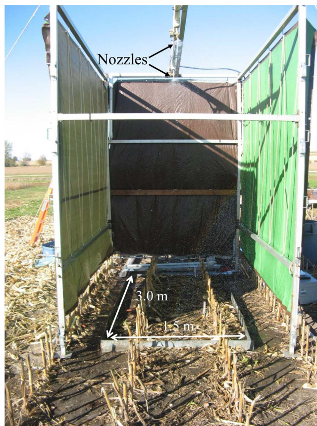
Fig. 1. Image of the twin-nozzle rainfall simulator installed on a no cover crop (control) plot depicting position of the plot boundaries spanning two corn rows with non-wheel traffic interrows. The tarp at the upslope end of the simulator was removed in order to obtain this image.
