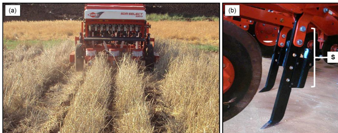
Fig. 1. (a) No-till seeders used to sow the crops in the experiment; (b) fixed shank opener that equipped the seeder for the sowing of soybeans ( Glycine max L.) and corn ( Zea mays L.), and, in detail (S), the set of screws that allowed to adjust the desired depth of operation of the shank.
