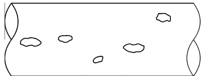
Fig. 1. Pipeline segment with multiple corrosion type defects.
