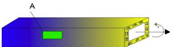
Fig. 3. Cracked beam under torsion.
