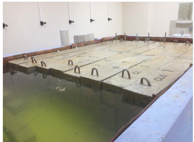
Fig. 1. Curing process of RC beams.
