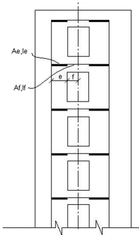
Fig. 1. Equivalent frame method as proposed by Schwaighofer and Microys.
