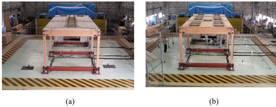
Fig. 1. Timber-RC hybrid building; a) laminated timber beam + RC slab diaphragm, and b) glulam + plywood diaphragm (CN75 @ 50 mm nail spacing).
