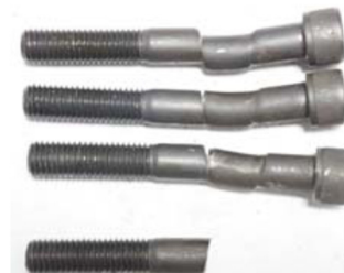
Fig. 2. Shear failure of bolt shank of SCBB.
