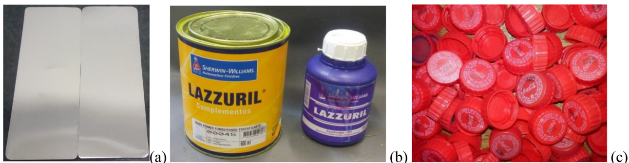
Fig. 2. Aluminium skins (a), Wash Primer components (b) and disposed bottle caps (c) used for sandwich panel manufacturing.
