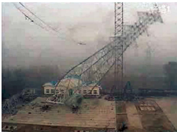
Fig. 1. Tower Collapsing During Full-Scale Test.
