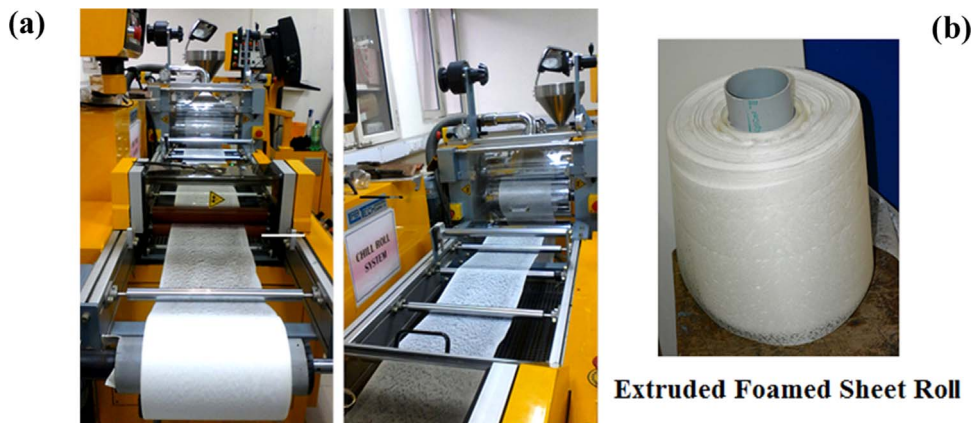
Fig. 1. (a) Pictures of continuous extrusion foaming of polymeric sheet (b) Extruded polymer roll.
