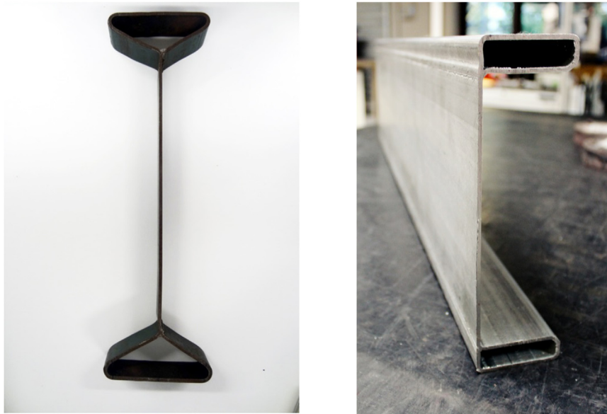
(a) Triangular Hollow Flange Beam
