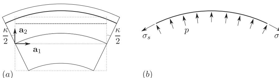
Fig. 2. Deformation of the beam segment under pure bending (a). Stress on the generic fiber plus radial pressure (b).
