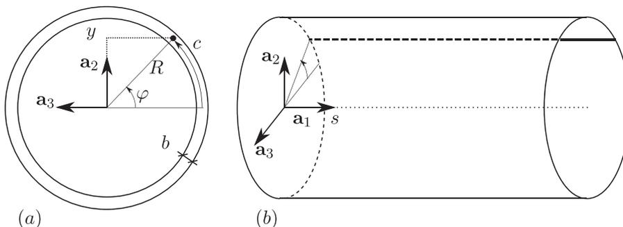
Fig. 1. Pipe beam: (a) cross section, (b) beam with a generic longitudinal fiber highlighted.
