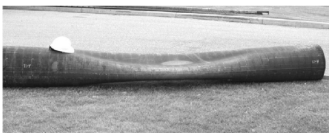
Fig. 1. Photograph of a 20-in., × 80 pipe collapsed under external pressure (courtesy C-FER Technologies) [23].
