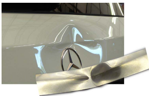
Fig. 2. An inverted strip compared to a “dent” in a vehicle body. Note the similarity of vertex shapes lying on the original crease lines.
