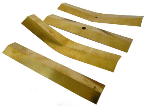
Fig. 1. Creased strips with and without a hole in their initial and inverted states. They are made from copper beryllium of thickness 0.1 mm, are 50 mm wide and 200 mm long.
