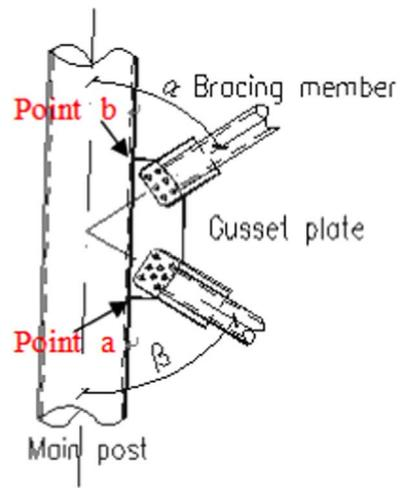
Fig. 3. Configuration of tube-gusset joint.
