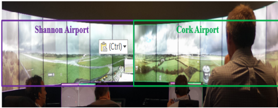
Fig. 1. The Remote Tower Centre located at Dublin Airport in excess of 100 miles away provided air traffic services for both Cork and Shannon airports.
