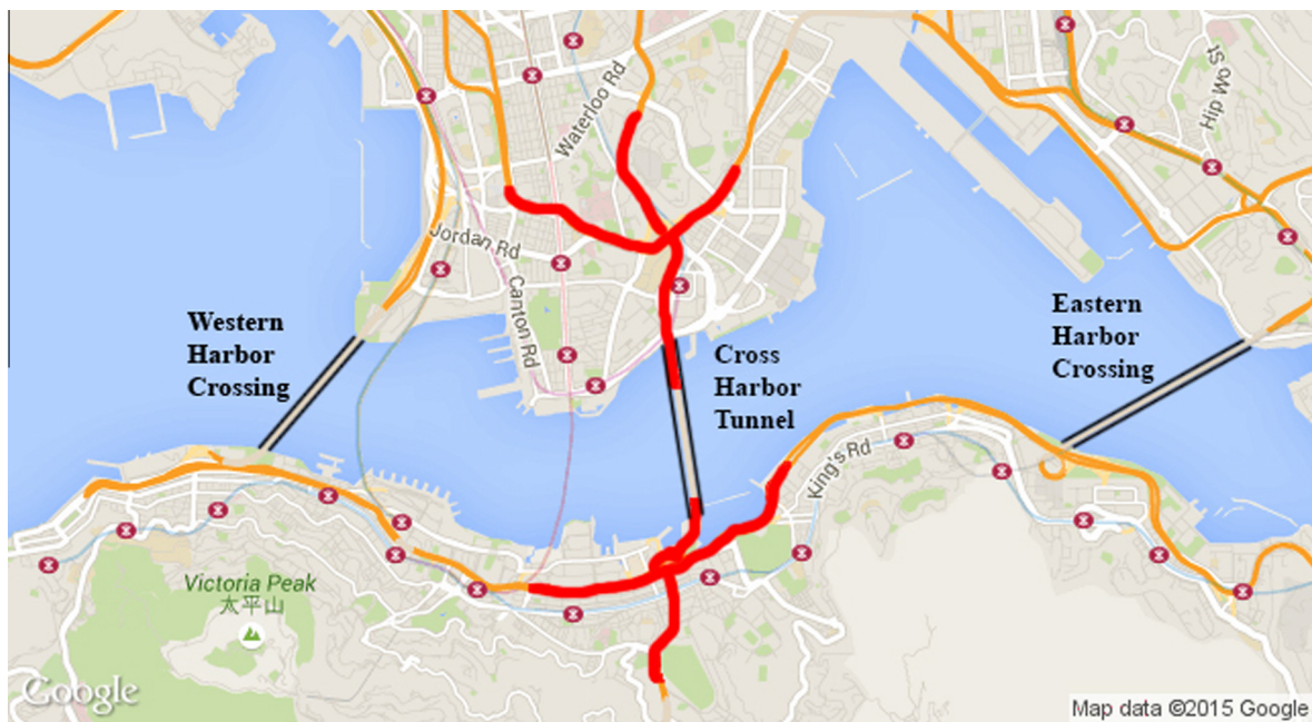
Fig. 1. Congestion problem of the Hong Kong Cross Harbor Tunnel, with the red line denoting the queue observed during daily rush hours on the tunnel's connecting roads (Wilbur Smith Associates Limited, 2010). (For interpretation of the references to colour in this figure legend, the reader is referred to the web version of this article.)
