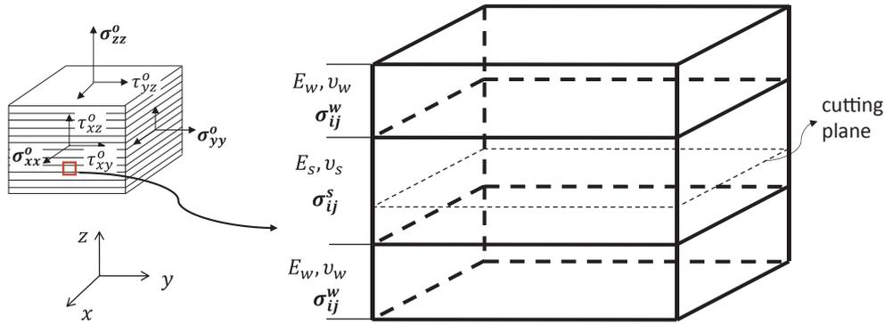
Fig. 1. Schematic diagram of interbedded strong and weak layers.
